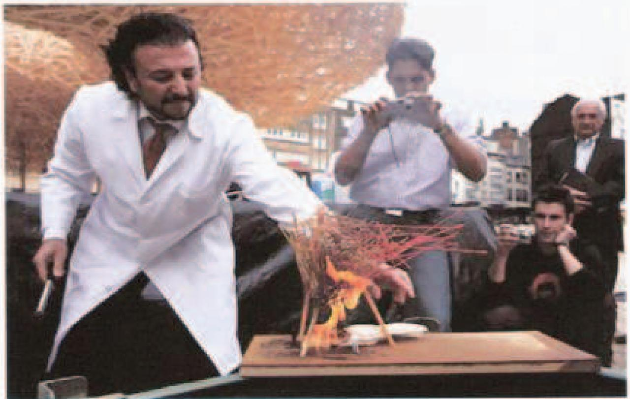
After being protected, the prototype was impregnated with gasoline and fired, but it could not be burned
