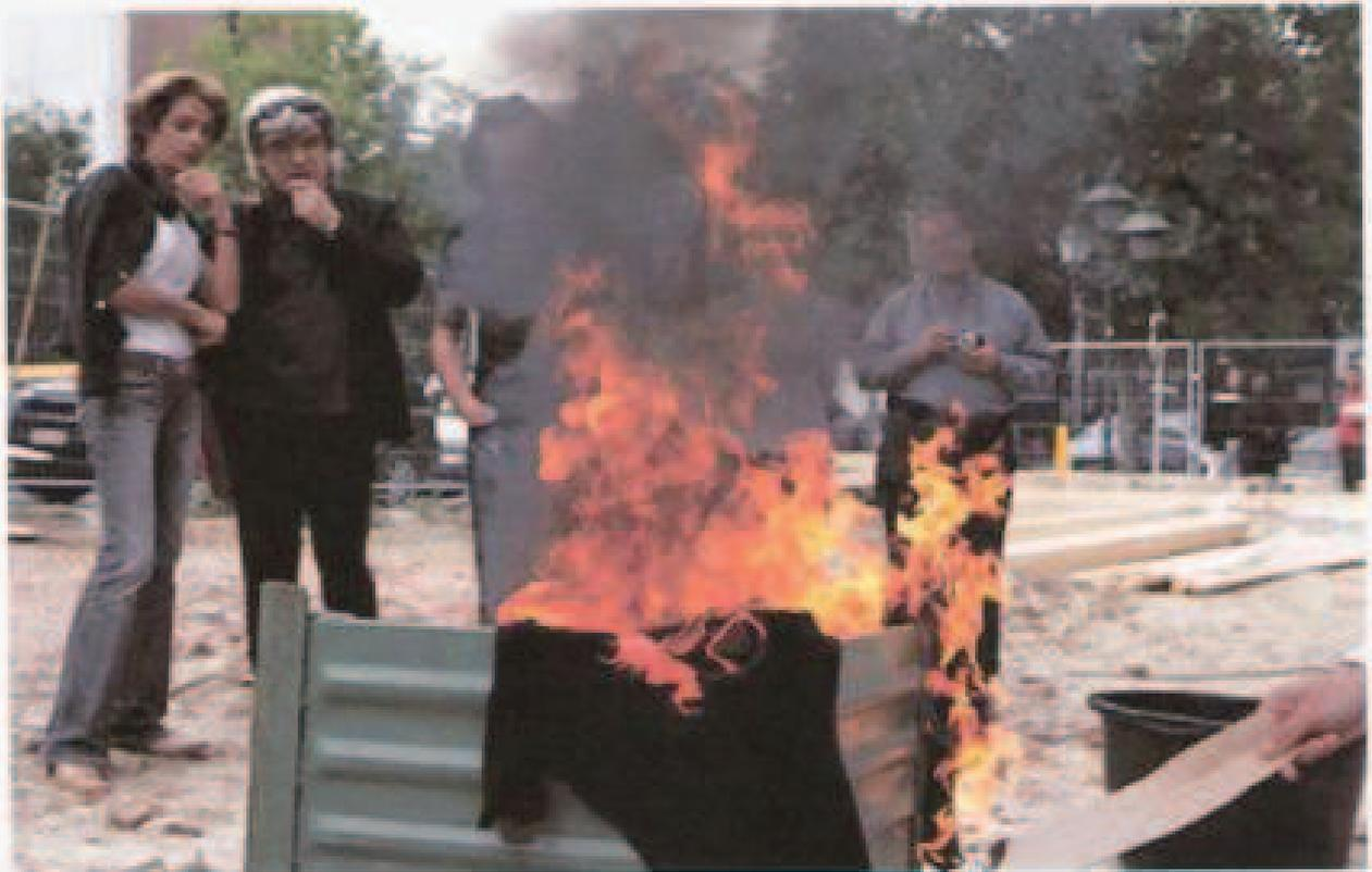
AyDo AquaElix Flame Safe showing another aspect of its performance. On the back one t-shirt was first protected with the Flame Safe, after wet with abundant gasoline and finally fired. The piece remained intact after the gasoline was completely burned. The t-shirt in front on the picture was first wet with regular water, after with gasoline and finally fired. The piece was completely reduced to ashes,
