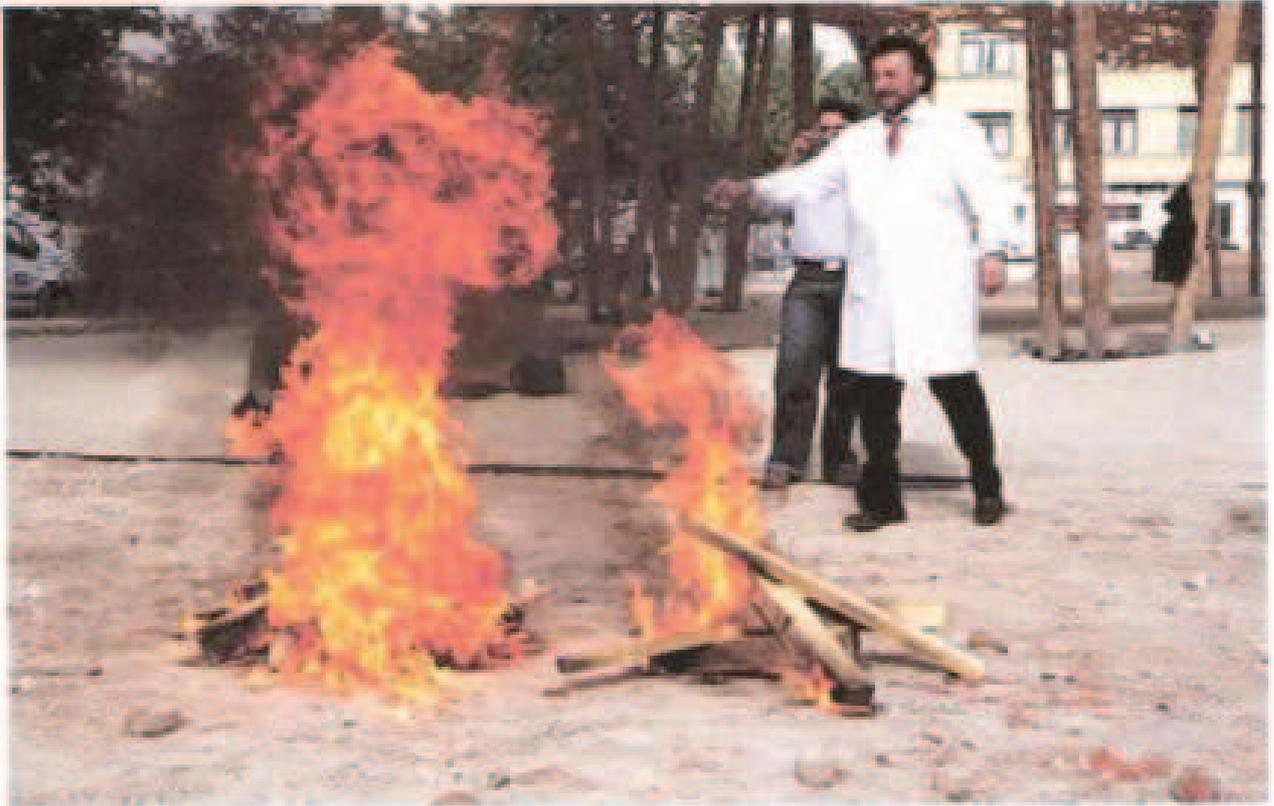
Samples of the wood used to build the structure of the Cityscape were taken to demonstrate the effectiveness of the AyDo AquaElix Flame Safe. The pile at the right was protected and as you see it doesn't burn. The pile to the left was not protected and the wood was completely burned. Notice the difference in the flame of both piles.
